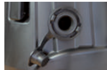
C-pipe connection for wastewater
